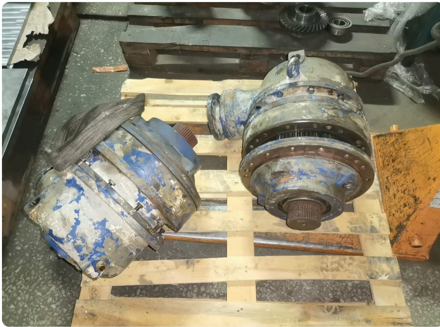
Gearboxes received for overhaul
