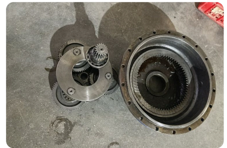
Planetary stage opened for inspection
